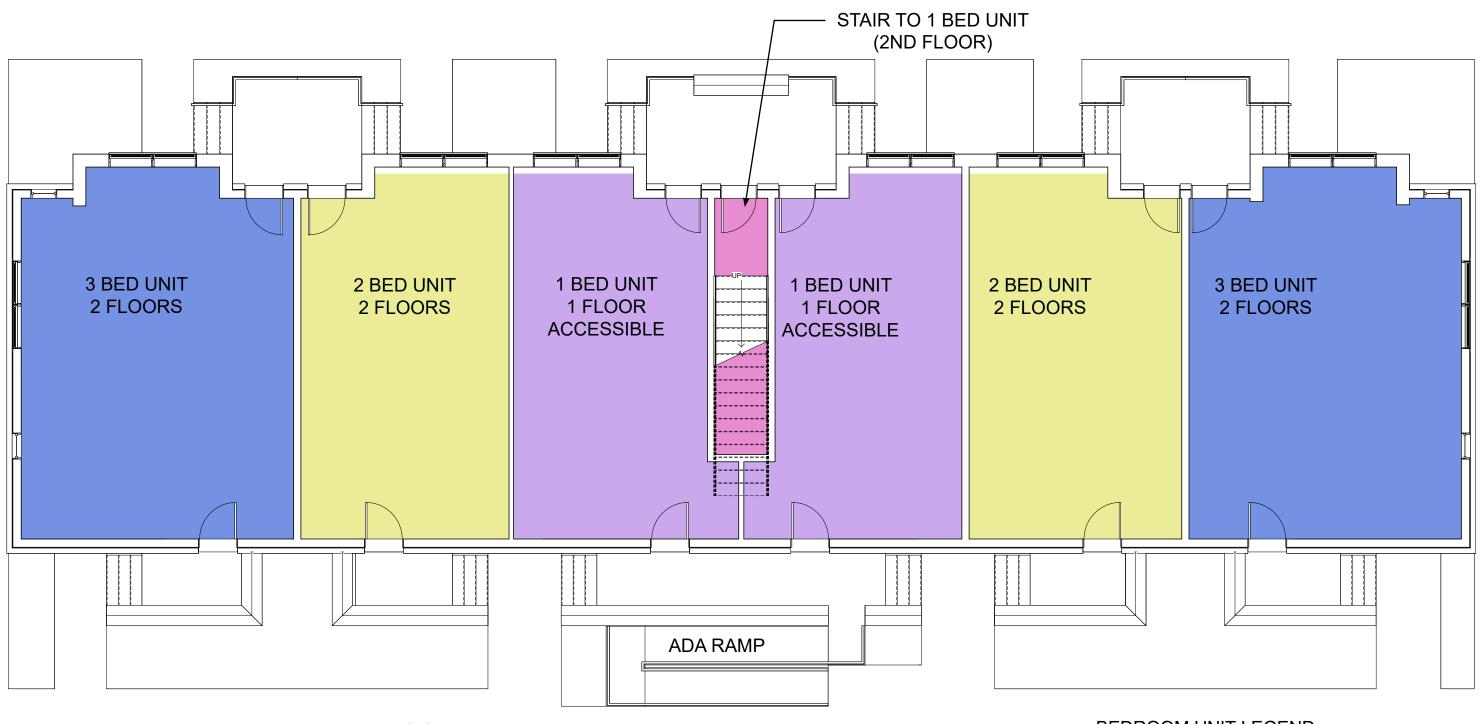
UNIT FLOOR PLAN SCALE: 1/8" = 1'-0"
