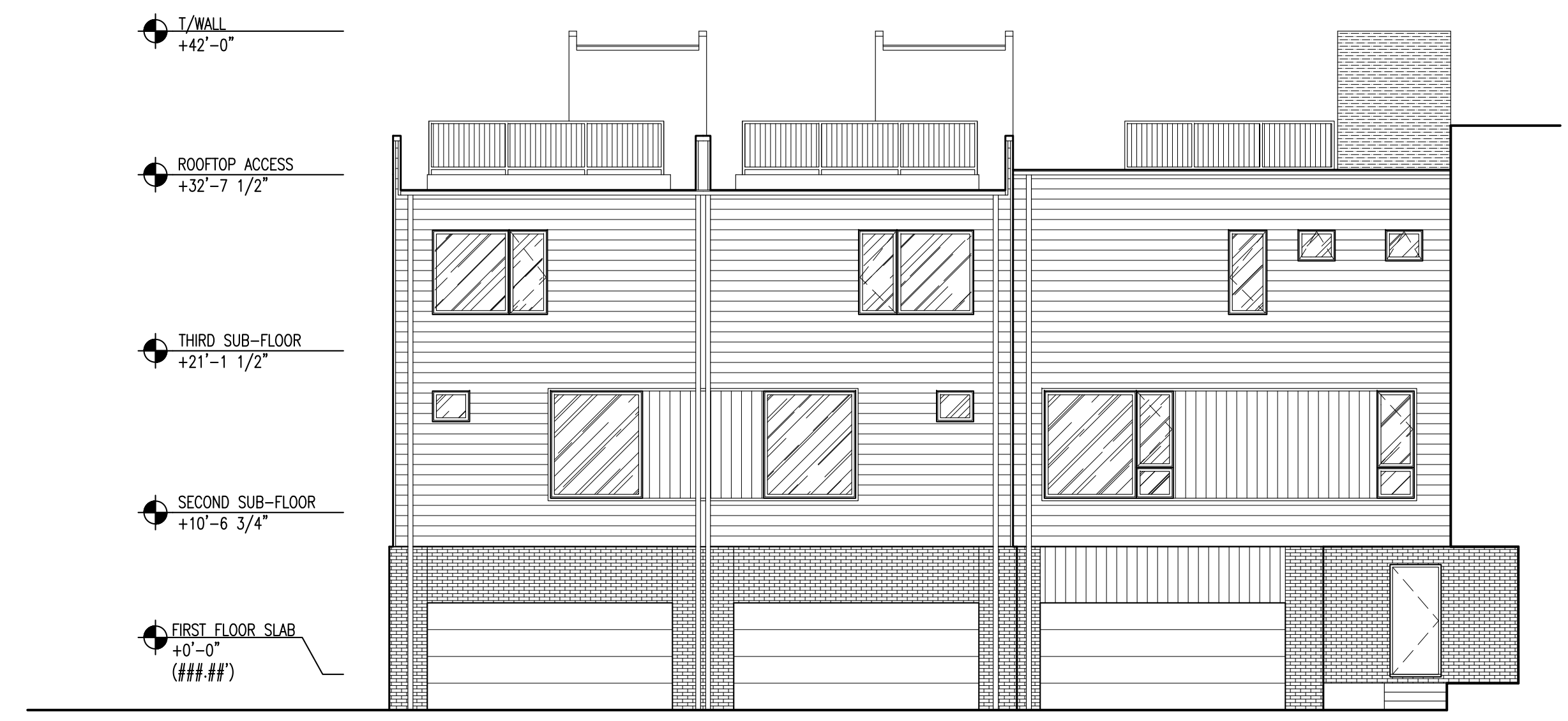
2 EAST ELEVATION - BUILDING 4 A202 SCALE: 1/8" = 1'-0"
