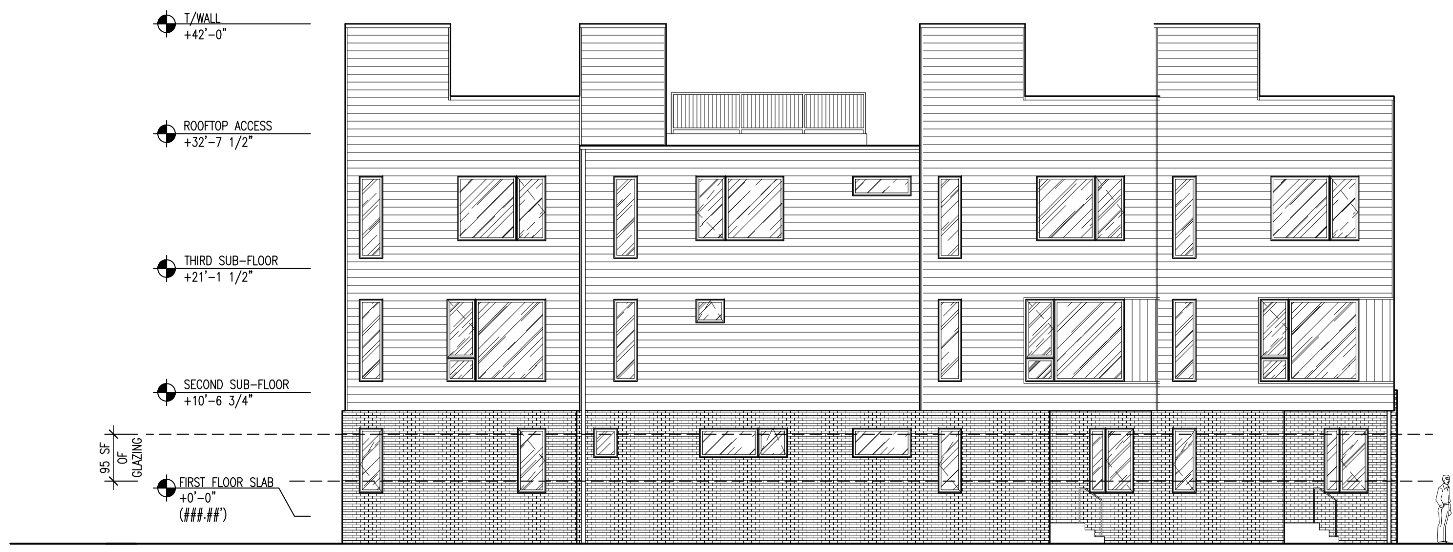
1 WEST ELEVATION - BUILDINGS 3 & 4 A202 SCALE: 1/8" = 1'-0"
